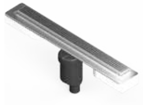
Pro-Line Shower Channel with Perforation with Removable Trap Vertical Outlet 50 mm Capacity 48 l/m Brushed Stainless Steel
